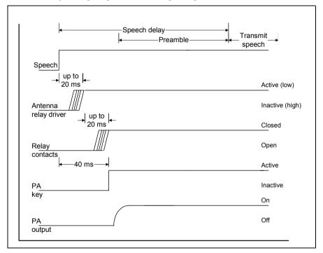
Antenna relay timing diagram for the beginning of an over
