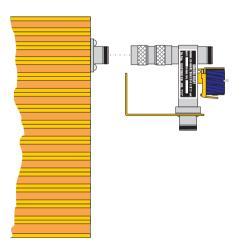
3. Secure the antenna relay bracket by fitting the supplied M3 x 8 mm screw through the bracket to the PA chassis.
