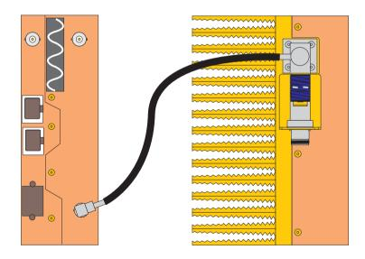
5. Connect up the antenna relay, as follows. Plug the DB9 connector to the DIG socket on the reciter. Connect the other wire to the +ve output of the auxiliary power.
