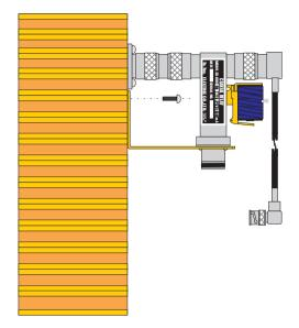
4. Fit the supplied cable (N-type to BNC) from the antenna relay to the receiver RF input.
